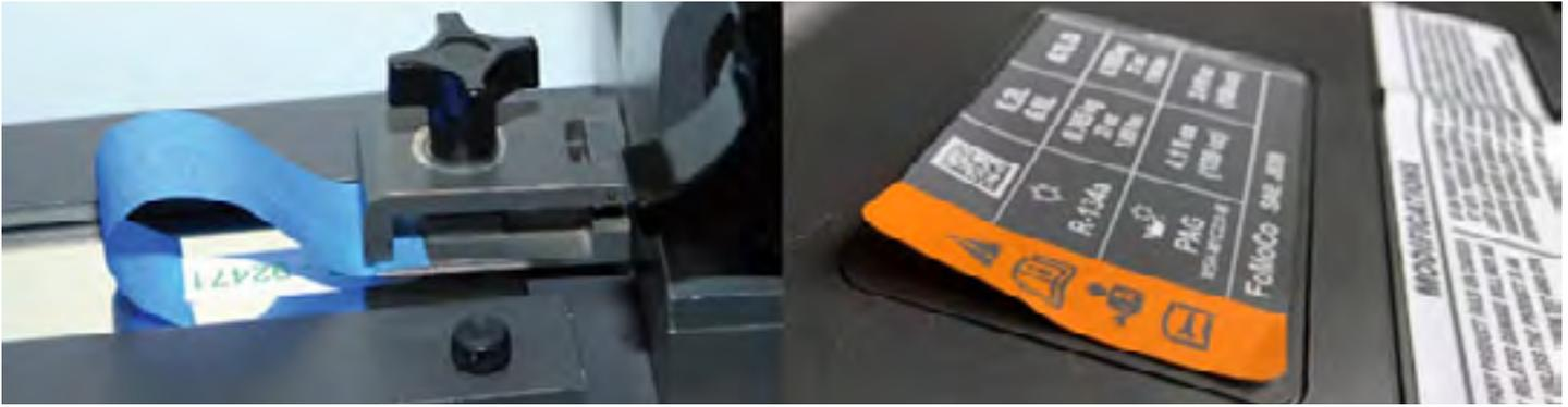
Peel Strength Test shown on Stainless Steel (left photo). Automotive Grade Permanent Pressure Sensitive Adhesive Label on polypropylene (right photo).
