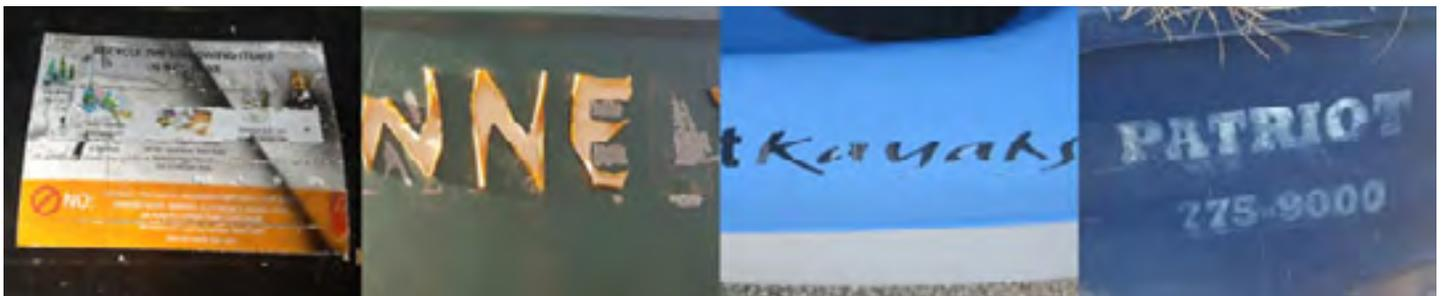
(Failed labels on polyolefins shown left to right: In Mold Label (IML), Pressure Sensitive Adhesive Label, Screen Printed Ink, Hot Stamp Foil).
