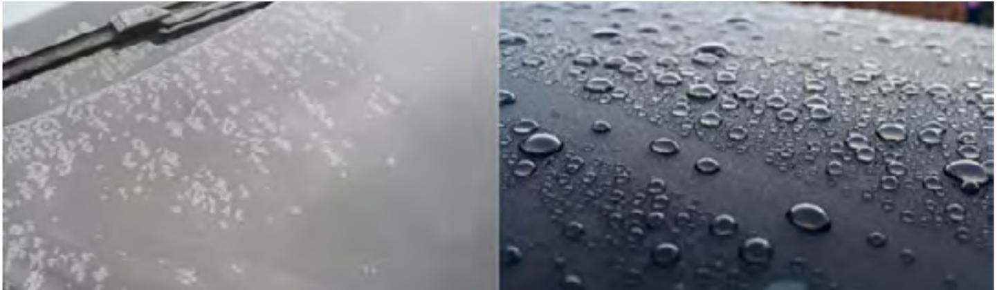
Wetting out of rain water on high surface energy vehicle (left photo). Beading of rain water on waxed low surface energy vehicle (right photo).
