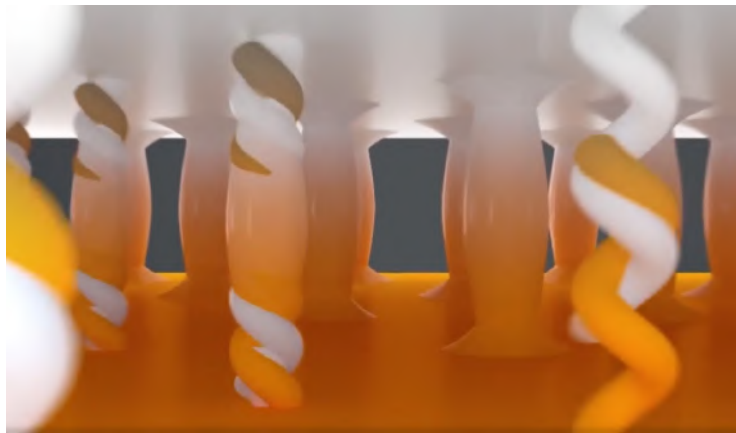
(TOP - Fusion Label, BOTTOM - Polyolefin Product, MIDDLE - "Fusion Reaction") Simulation of Polymer Fusion Label fusing to Polyolefin Thermoplastic Product
