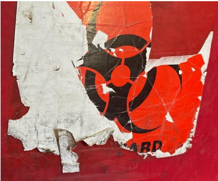
Failing adhesion-based biohazard label applied to HDPE.
