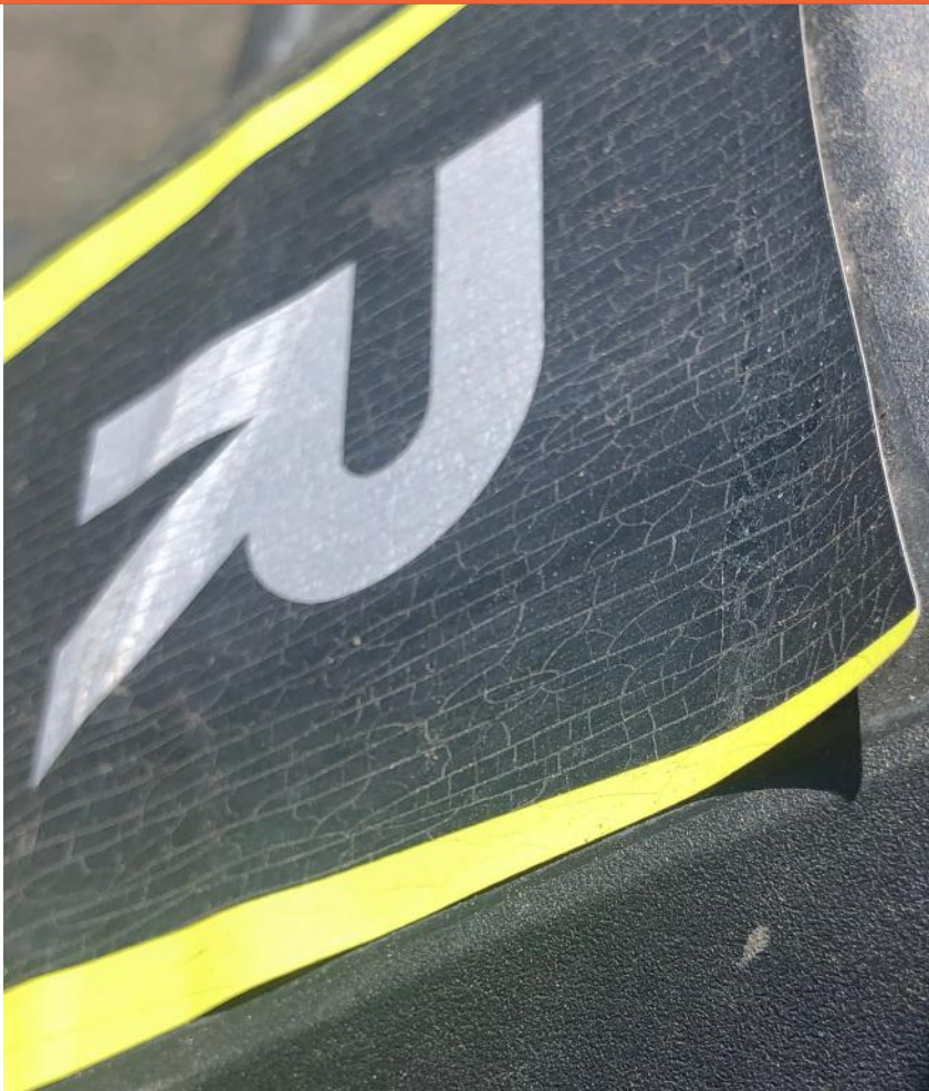
Failing adhesion-based durable Brand Recognition label applied to brand new Ryobi Brand LSE Plastic riding lawn mower component.
