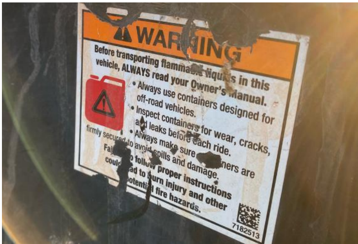
Failing adhesion-based durable label applied to offroad vehicle LSE Plastic.
