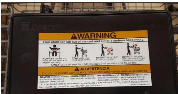
Polymer Fusion Technology label printed and fused to LSE Shopping Cart Seat Flap. Label is still in service at 6 years old.
