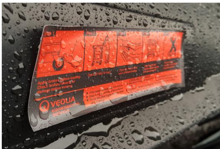
Failing adhesion-based durable label applied to LSE Plastic.
