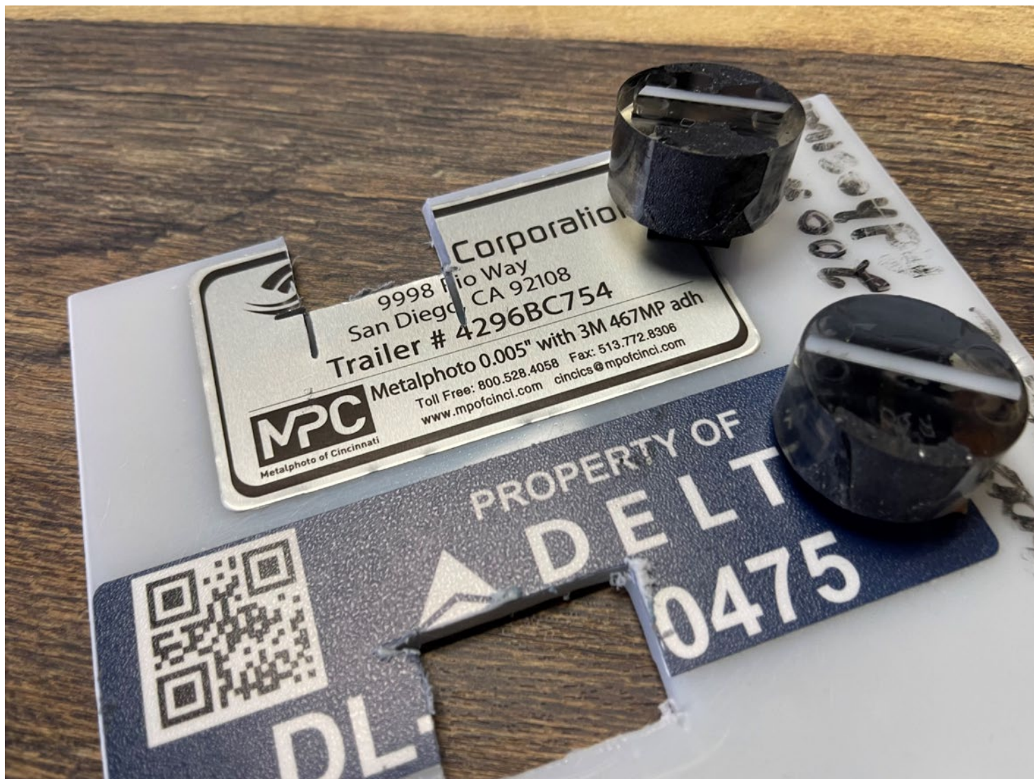
Pressure Sensitive Adhesive (PSA) Label Cross Section within Mounting Surface for SEM Analysis
