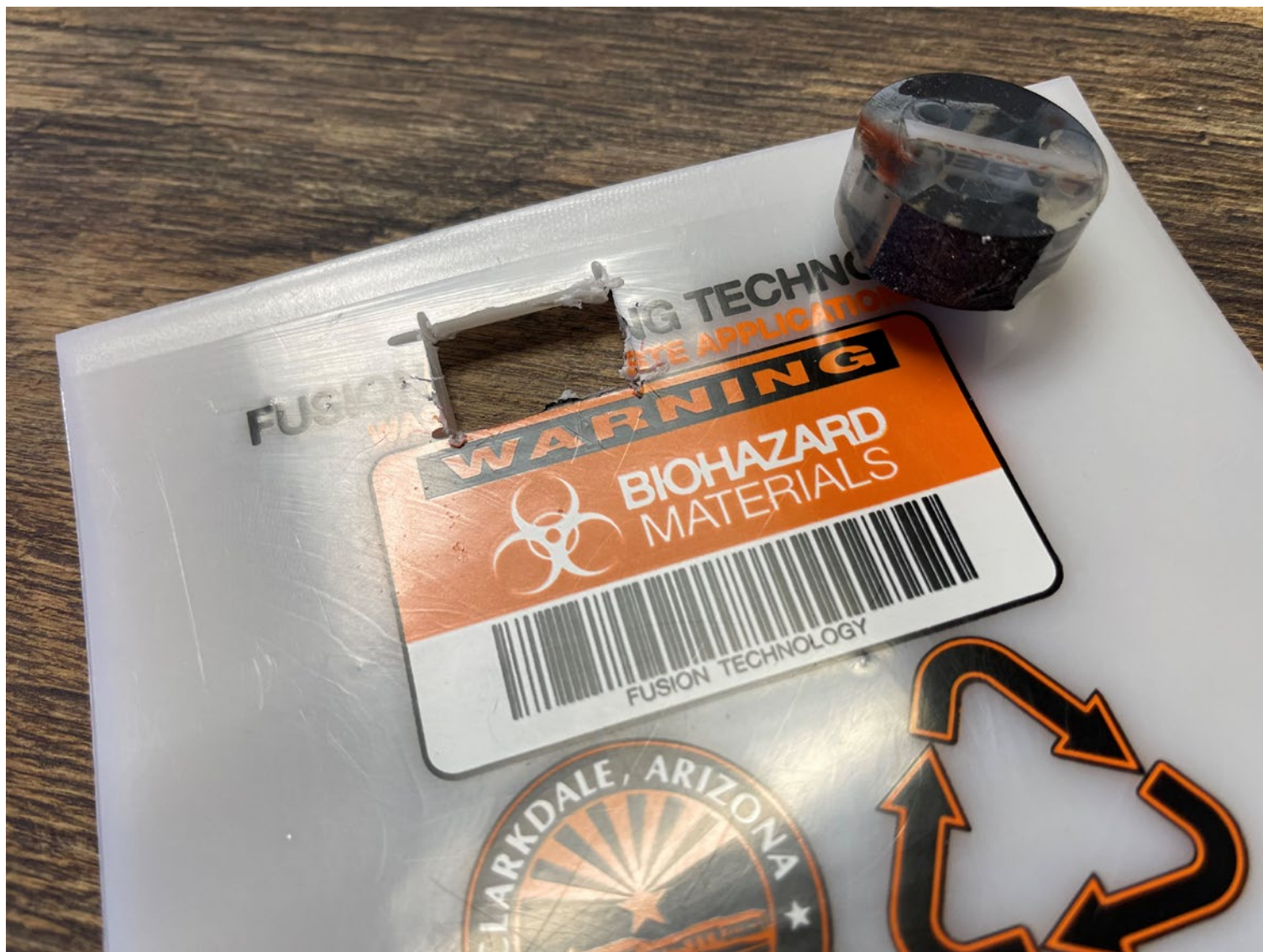
Polymer Fusion Label Cross Section within Mounting Surface for SEM Analysis
