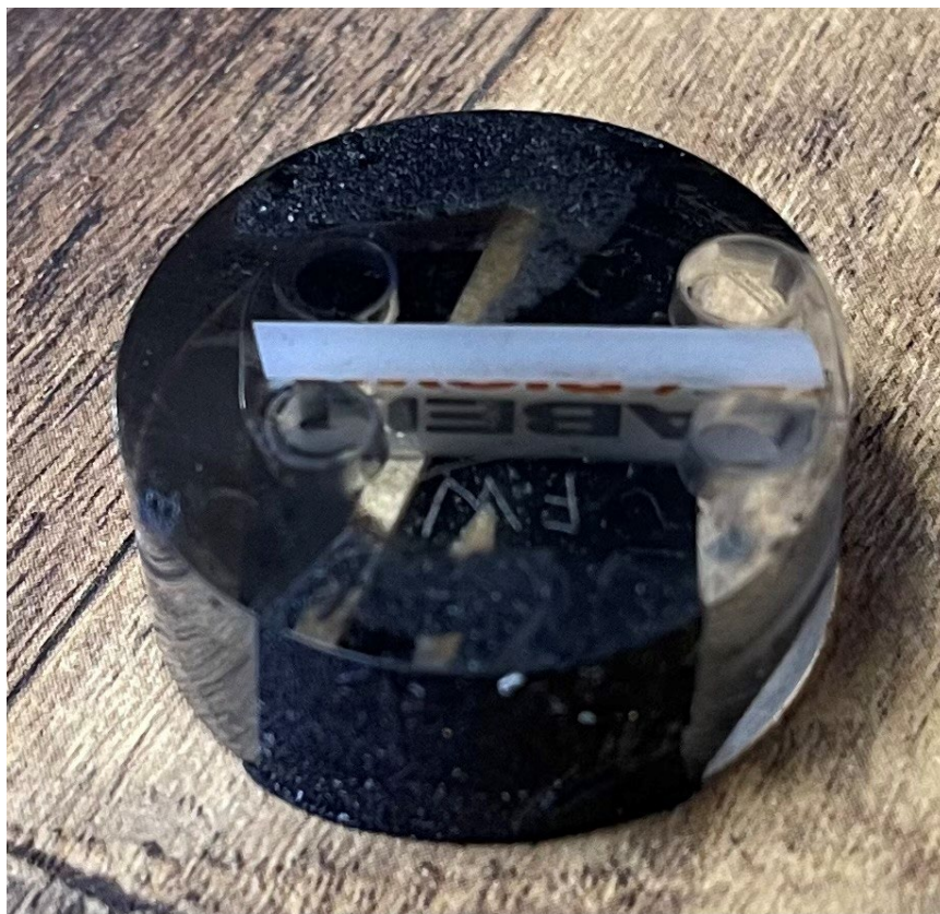
Label Cross Section within Mounting Surface for SEM Analysis
