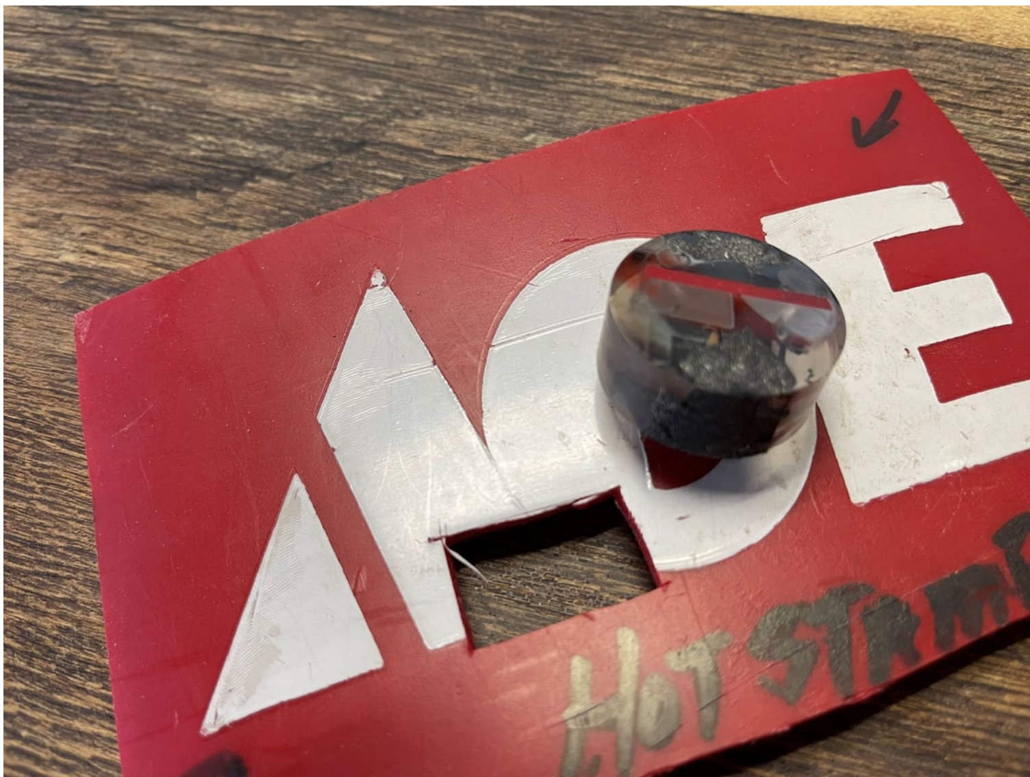
Hot Stamp Foil Label Cross Section within Mounting Surface for SEM Analysis
