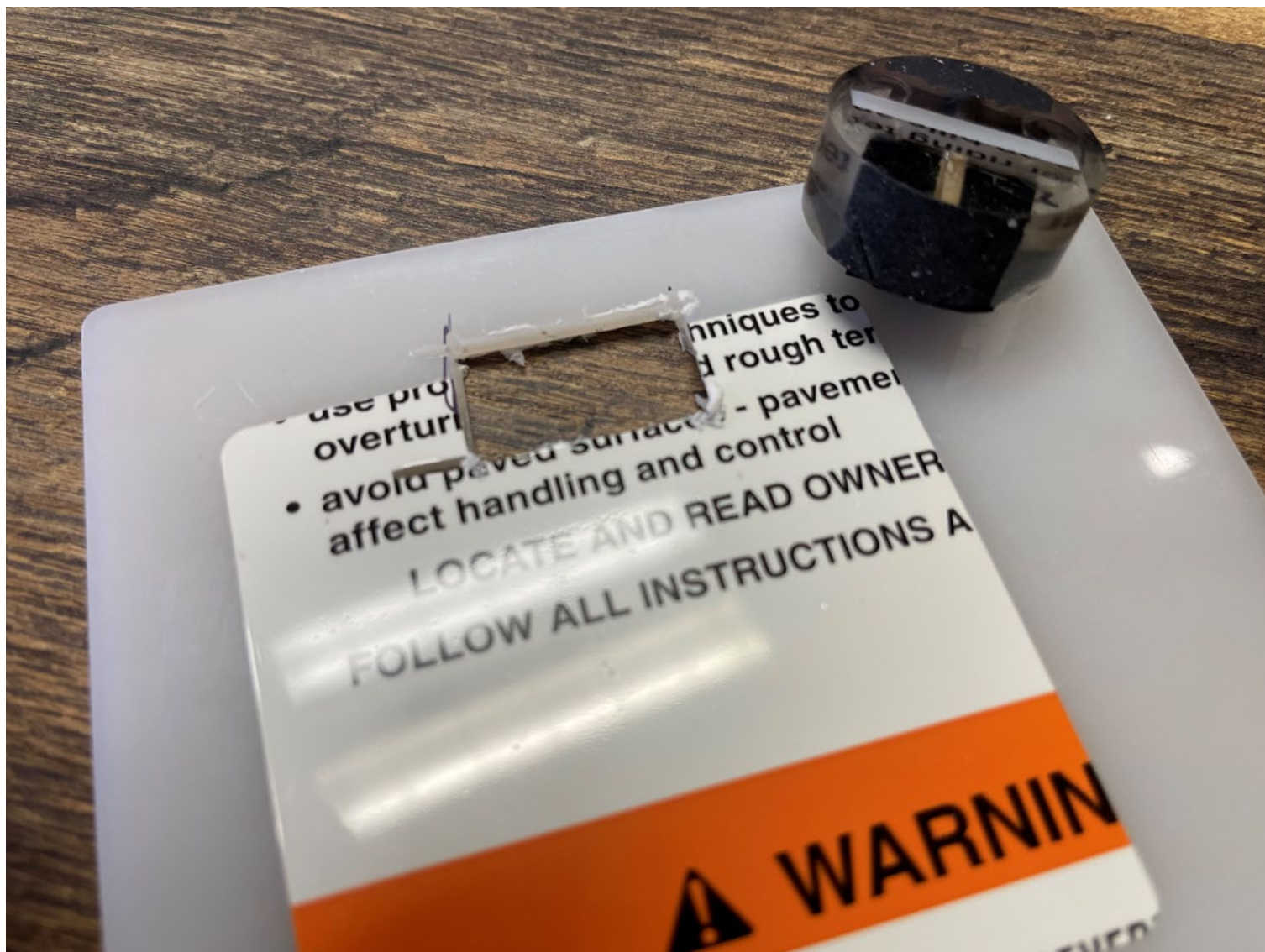
IML Label Cross Section within Mounting Surface for SEM Analysis
